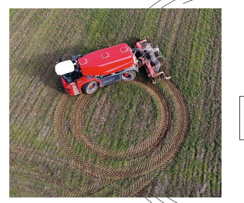
Pulling power, endurance and ground clearance are of paramount importance to us. This is why the new Quad is not only rugged and robust but also uses innovative design techniques to make it the strongest and lightest self-propelled vehicle in its class with a tight turning circle thanks to its sophisticated four-wheel steering.
