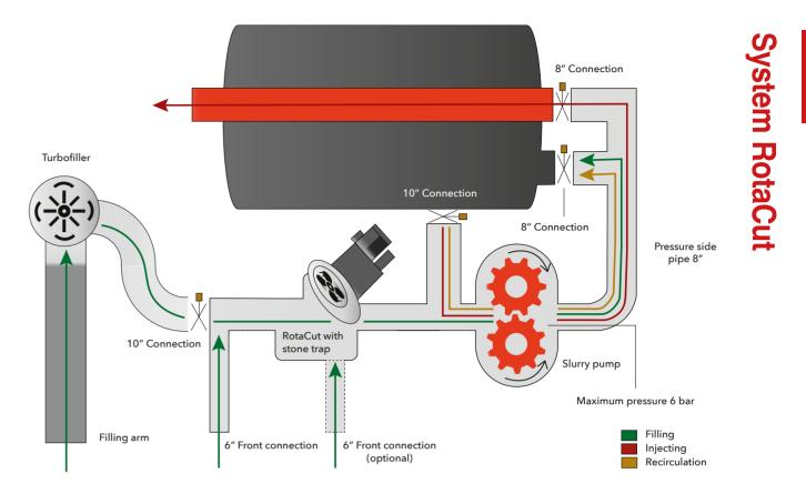
The RotaCut system o ers shorter lling times thanks to the Turbo ller used in combination with a Vogelsang RotaCut macerator, which shreds the bres and foreign matter, protecting the slurry pump from damage.
