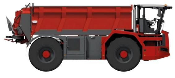
In addition to liquid manure (slurry) application, the Quad 550 was designed from the outset to spread solid too. Our knowledge and experience with the Trike equipped for solid spreading was applied to the four-wheeled chassis.
