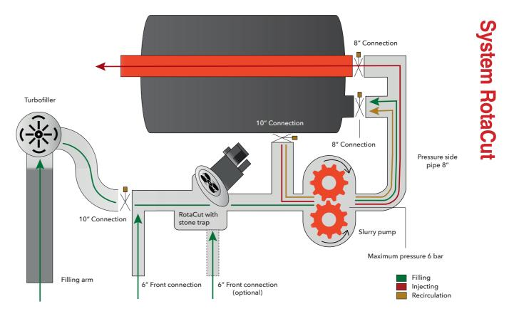
The RotaCut system offers shorter filling times thanks to the Turbofiller used in combination with a Vogelsang RotaCut macerator, which shreds the fibres and foreign matter, protecting the slurry pump from damage.
