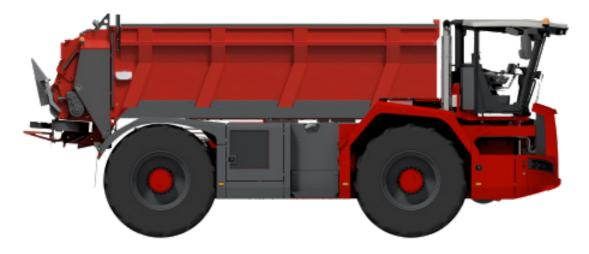
In addition to liquid manure (slurry) application, the Quad 550 was designed from the outset to spread solid too. Our knowledge and experience with the Trike equipped for solid spreading was applied to the four-wheeled chassis.
