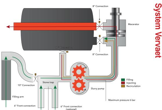
By placing the unique Vervaet cyclone macerator after the slurry pump resistance on the suction side of the pump is minimised. The pump works continuously, both whilst manure is being spread and during headland turns when it automatically switches to recirculation. During recirculation the chopper is constantly cleaned to prevent clogging. Thanks to this recirculation the system is constantly primed with slurry so that it reaches the target as soon as the application unit is lowered into work.
