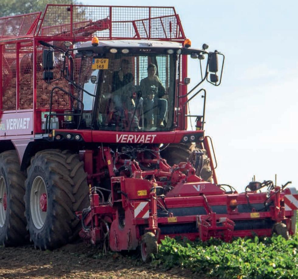
Just like the smaller Q series, the Beet Eater can be equipped with hydraulic levelling. This unique technology keeps the superstructure of the harvester level as circumstances demand. If it is hilly, for example, but also on the slopes of ditches. The levelling provides extra stability and the pressure on the ground is spread more evenly.
