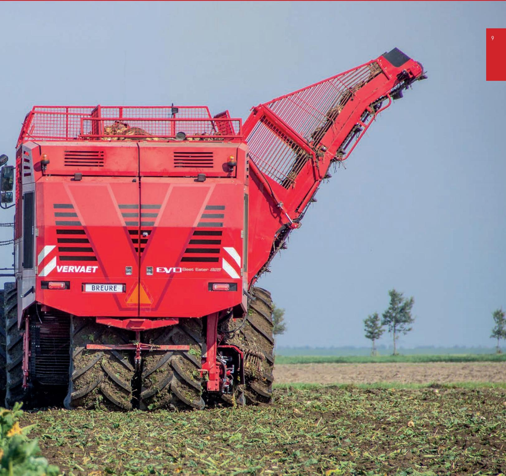
This principle is also unique to the nine-row, in particular, because here the tyres just make one track. Combined with the excellent weight distribution, it's a monster with huge capacity that nonetheless takes account of the soil structure.
