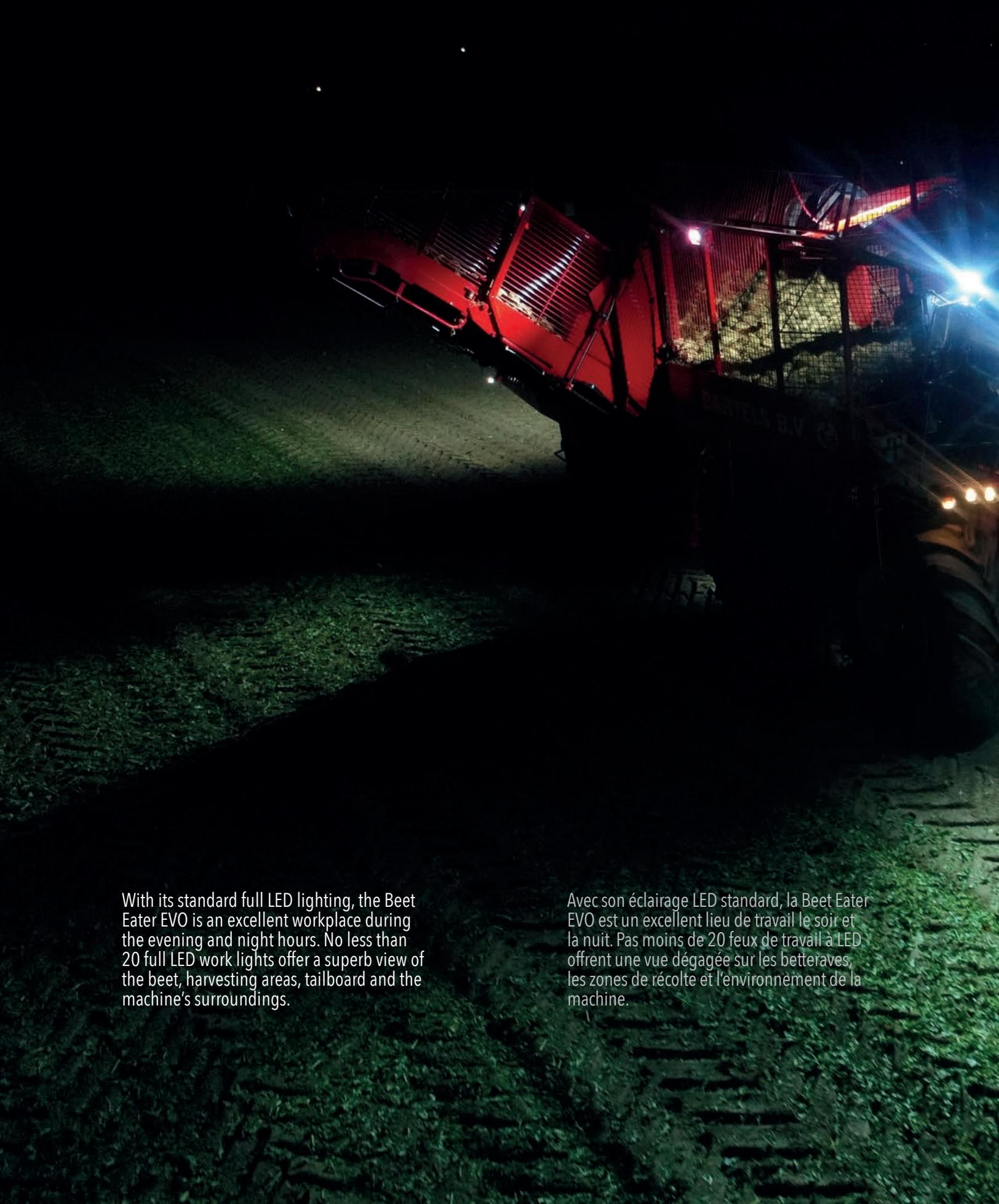
With its standard full LED lighting, the Beet Eater EVO is an excellent workplace during the evening and night hours. No less than 20 full LED work lights offer a superb view of the beet, harvesting areas, tailboard and the machine's surroundings.
